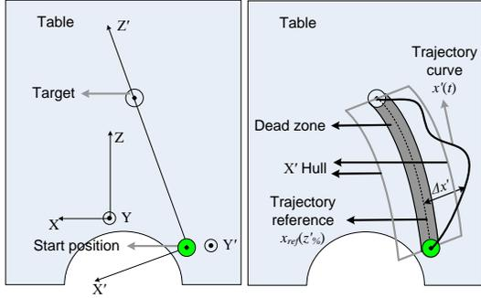
**Figure 3.** Hand trajectory along the table plane. Left: Global coordinate system XYZ and local coordinate system  $X'Y'Z'$ . Right: the reference trajectory, dead zone and the hull.
